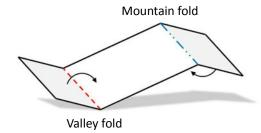
Score all the valley and mountain folds using either the corner of your ruler, a butter knife, scissors, or pen that's run out of ink. Fold all the scored lines well to create sharp folds.
