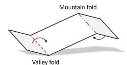
Score all the valley and mountain folds using either the corner of your ruler, butter knife, scissors, or pen that's run out of ink. Fold all the scored lines well to create sharp folds.
