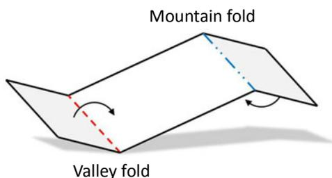
Score all the valley and mountain folds using either the corner of your ruler, a butter knife, scissors, or pen that's run out of ink. Fold all the scored lines well to create sharp folds.
