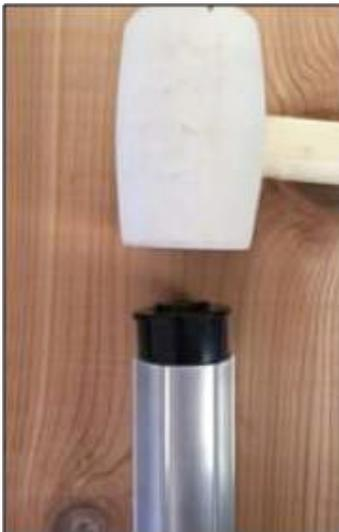
After smoothing out the cut end of the Roller, line up the End Cap on the Rollers. Using a rubber mallet, gently tap in the End Cap into the Roller, fully, ensuring it stays level as its being inserted.
