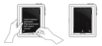
**Step 2:** Take the iPad Spacer and install it into the end of the Padcaster insert at the bottom of the iPad. Work the spacer into one corner first, then press the spacer down while working it under both center-tabs of the insert and finally, the lower corner.
