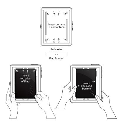
**Step 1:** Starting with the camera lens side, press the iPad into the insert corners. Work the edge on the insert around the outside of the iPad until the insert perimeter completely covers the outside edge of the iPad. **NOTE:** You can apply some force to work the iPad in. The fit should be tight and you will NOT break the iPad glass.
