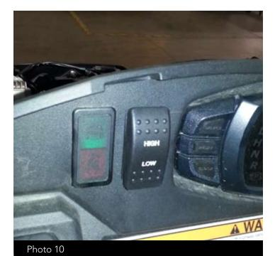
10. Locate the heater switch adhesive template and place it on the dash as shown (**Photo 10**) and cut out the black line with a sharp razor knife. (**Photo 11**)
