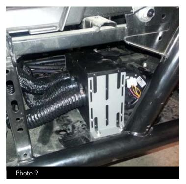
9. Route the heater's wire harness from the heater unit, under the floor and into the area behind the dash. Use the protective split loom to protect the wire and secure to the previously ran heater hoses in steps 3 & 4 using wire/zip ties. (**Photo 2**) shown without split loom for visual identification.
