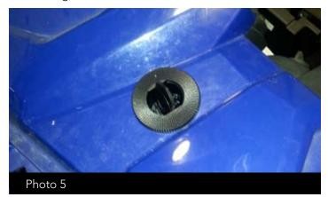
**NOTE:** The positioning of the vents in the seat bases and dash are critical to avoid cutting into wires, hoses, etc. Always check clearance behind any area to be cut or drilled.
