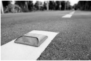
A cat's eye is a small safety device in the road. The driver needs to see the middle of the road at night. When a car's headlights shine on a cat's eye, it lights up.
