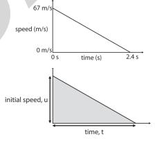
Here is the speed / time graph for the jet's motion.
