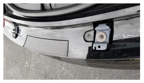
5) (Wing will come with Brackets attached with Bolts, Remove brackets from Wing) Install brackets as shown with factory nut removed from before, do not over tighten, leave the brackets loose enough to be able to adjust wing once lowered into position. Will need 2 people to do this step.
