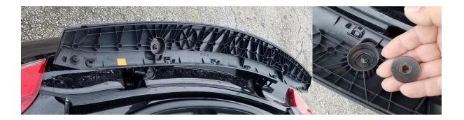
3) Once Top cover is removed, remove the 2 nuts holding the bottom base Cover, Remove Cover, Save the 2 nuts to attach Wing Brackets with.
