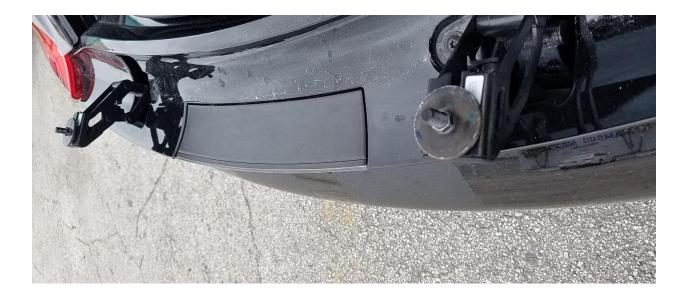
4) If the height of the spoiler need to be adjusted, these are the Nuts that can be adjusted to correct the height.
