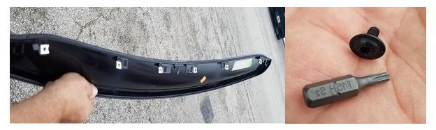
2)Once raised – Remove screws with T15 Torx Tool, along the front edge and remove spoiler cover
