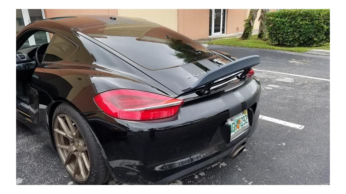
6) Install ducktail onto brackets with the 4 bolts that where provided with the wing. Once wing is tightened, have one person lower the wing slowly using the button from the console while you adjust the wing from left to right, and check Gap against Lid. Once Wing is centered, raise wing back up and carefully remove wing, without moving bracket location. Tighten the nuts from Step 5. If the height needs to be adjusted, refer to step 4. Install Wing onto Brackets again, check fit. DONE!
