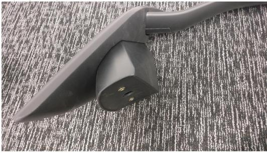
8.- Finish assembly the spoiler together. Ready to install the spoiler using the last 4pcs gold screws.
