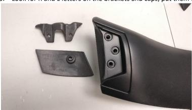
4.- Align the bracket with the side blade, use the 3pcs silver screws on each side. Do the same on Right and Left side.
