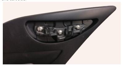
5.- Use 2pcs of the gold screws to secure the side blade bracket with the center blade. (Do not over tight the bolts)
