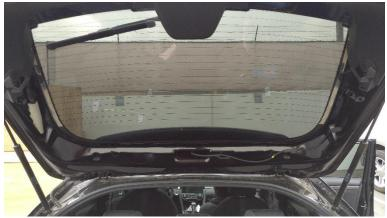
11. There are two bolts need to remove under the handle. Do the same on each side. Then the whole panel should come off with just clips.
