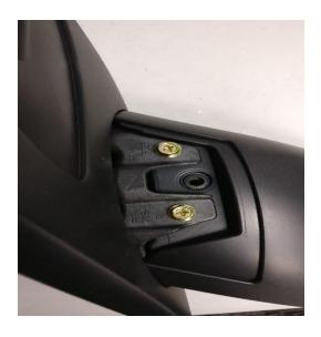
6.- At the end use the Hex screws secure the cap cover over the bottom of the bracket.
