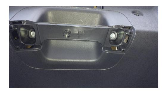
12. Locate the position of the spoiler holes need to be drill. We suggest use a small drill bit to drill first. Then place the template of the hole to align the position.
