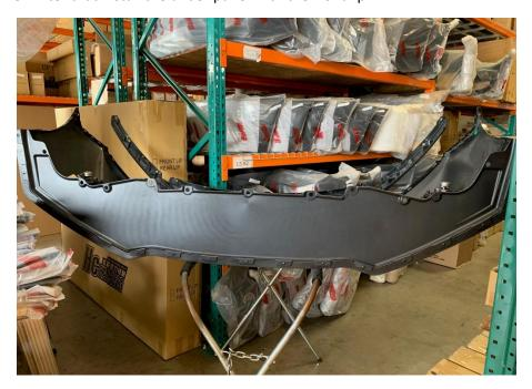
9.- Attach the under panel to the front lip. Using screws. Note do not puncture the screws through. There are two spot cut out does not need to be screw in.
