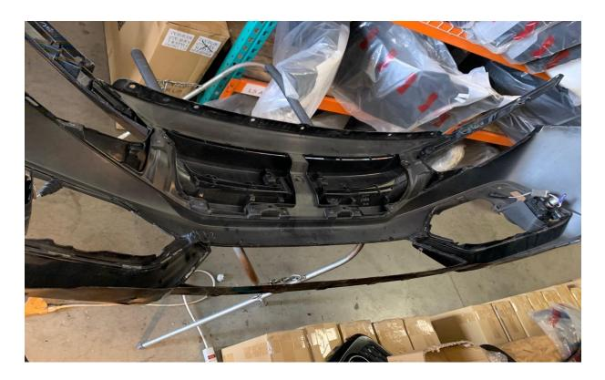
6. Install the new grill on the bumper. Reuse the original screws and put the grill into the bumper tabs.
