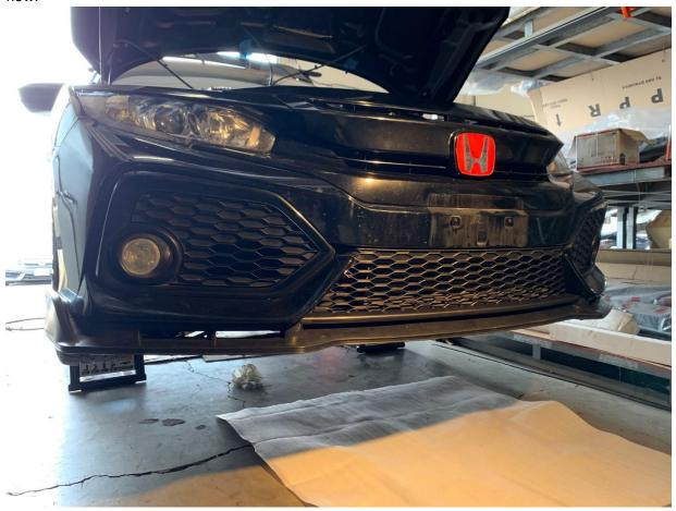
11. Next step is to attach the under panel to the bottom of the car using original tabs and bolts. Some holes might not require to use.
