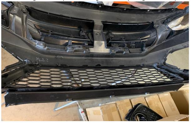
7. —Install the Type-R front lip on the bumper next. By align the mounting point with the grill. Then tight down the lip by using supply screws. Do not over tight by power tools. Make sure the screws not puncture through.
