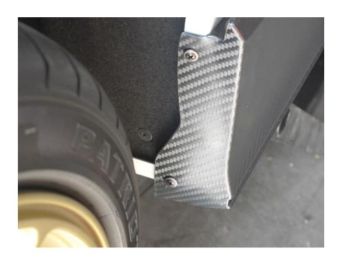
9.- Now we are moving down to the bottom of the side skirt extension. We need to secure four tapes on the bottom with the supply screws.
