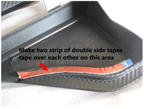
6.- Install the front of the side skirt extension on the car first. Make sure no gap with extension and oem side skirt. Remove the double side tapes then push it toward the oem side skirt. While pushing in use a self tapping screw and a washer, screw it throught the gold bracket in from the bottom to
