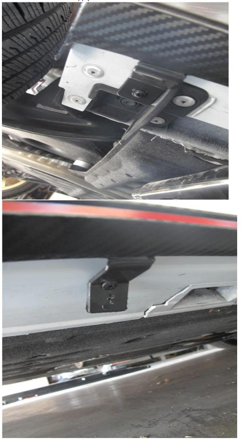
10. When all tapes were screw in then you are done with the installation on the Type-r Side Extension on one side. Use the same steps on the other side skirt.
