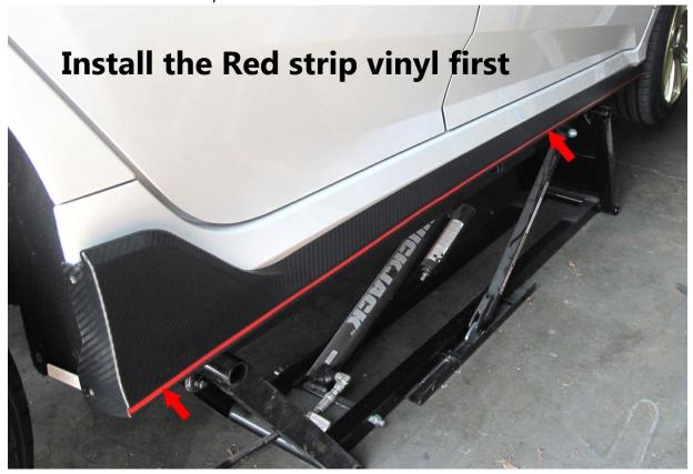
3. – Before assembly the side skirt on the car. Clean side skirt inside tape area with alcohol and clean out any dust or oil on the car.
