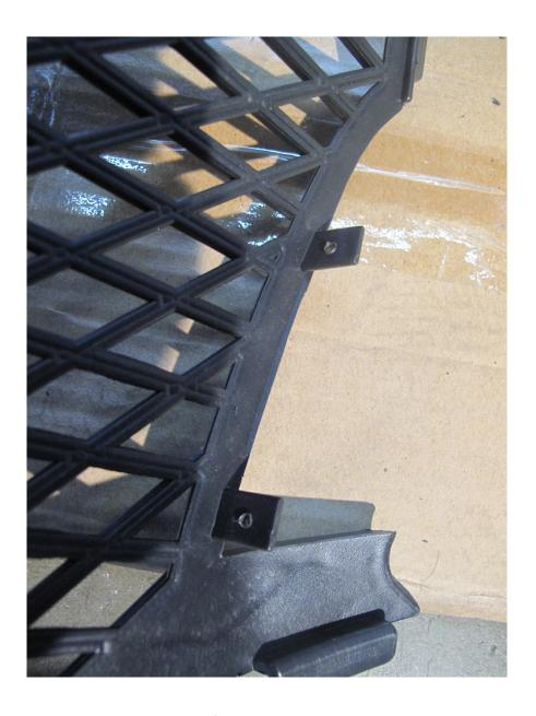
8. Insert the Type-R carbon fiber pattern lip onto the bumper. There are 8 tapes need to slide into the bumper slots.
