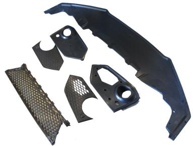
3. – First assembly the two foglight cover together. Foglight cover come in two part. Use supply screws to combine both together as show on picture.
