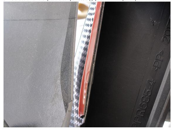
10. Each side of the front lip have a cross mark. Insert screw to secure the lip to the bumper.
