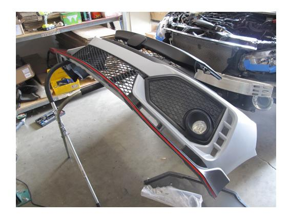
9.- Before screw on the lip to the bumper. Use supply double side tapes on picture show area.
