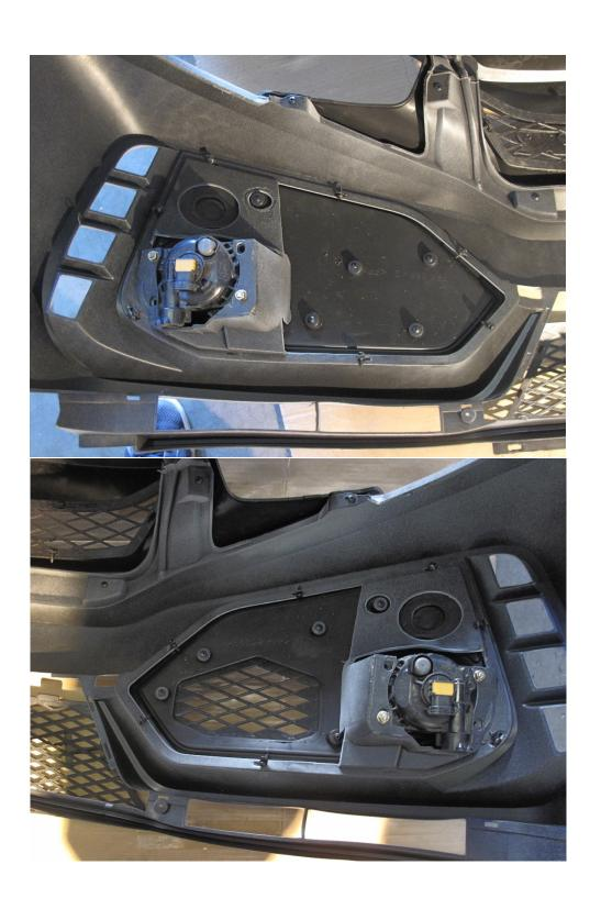
6.- Install the foglight cover back on to the bumper use screws to secure it on the tape where the pre drill holes are with the bumper. Show in picture.
