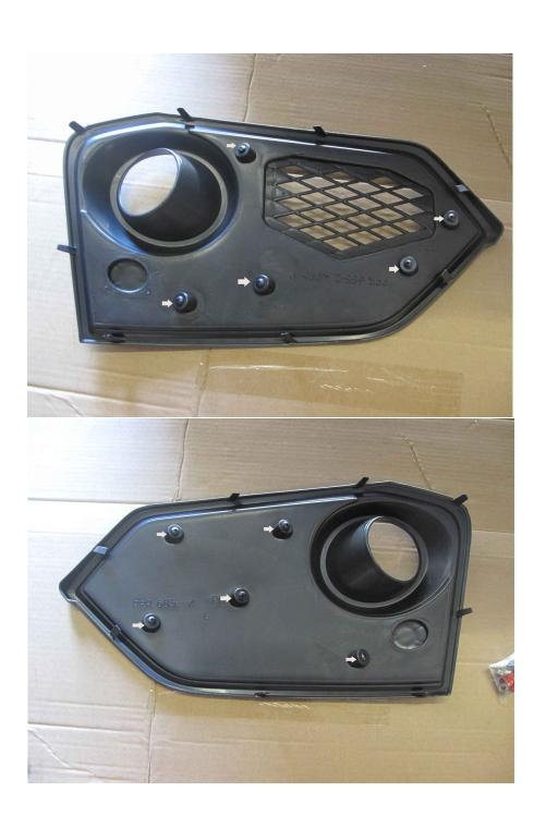
4.- Each foglight cover have eight taps around. Use a small drill bit or any shape object to make a small hole on each tap about 0.5cm from the edge. See show pictures.
