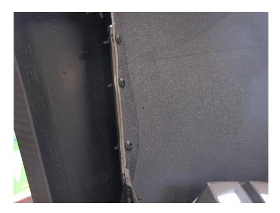
13. Next install the under panel on the bumper. Use 4 supply gold nuts and bolts to secure on side of the panel to the bottom lip. There are marking print on the panel to insert the black screws to secure the panel to the center of the panel to the lip.
