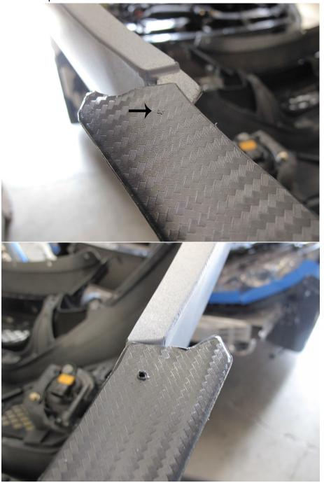
11. Next drill small holes on each tape when the lip fully insert to the bumper. In the center there are 6 tapes need to insert with the grill then use screws to secure it . Show on picture.
