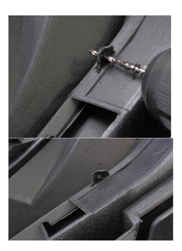
12. Use supply screws to secure the taps on the lips. There are two big size gold screws insert on the back of the bumper to the front lip toward center of the bumper. Then use a small drill bit to make holes on each area on the under side of the lip to the bumper. Show as the picture.
