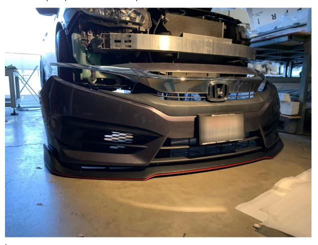
9.- You are ready to put the bumper back on the car now. Reverse the step from remove the bumper.
