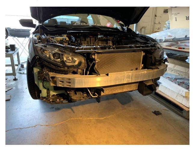
2.- Open the hood remove top radiator cover by remove all the taps first. Then unclip the headlight eyelid from the headlight. Remove all the screws secure the bumper on each side of the fender and bolts and taps on the bottom of the under panel. Then your bumper can pull right off the car.
