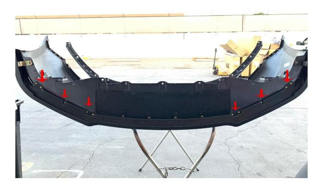
7. – Check fitment after finish install the lip on the bumper. Make sure to check on the red arrow area.
