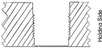
Prep the "holding" side and the "receiving" side as described in installation instructions. Using P/N AA03-004-004 insertion tool. Screw the IVB precision locator into the 1 1/4"-12 threaded hole until shoulder of IVB precision locator "bottoms" in the hole or until face of locator is flush with "holding" side.
