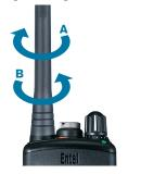
To attach, carefully align the antenna with the socket. Screw in the antenna and clockwise (taking care not to cross the thread) until it is seated firmly with the accessory cover's rubber ring between the antenna and the top of the radio (A).
