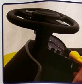
3. Put the screws into the set plate and use them to screw the screwdriver tightly.
