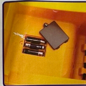
5. Remove the seat plate and use the three-section 5 battery. The corresponding positive and negative poles are installed.
