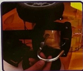
1. Pass the steering shaft from the bottom of the body. The hook is also stuck in the plastic hole.
