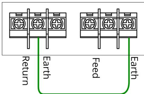
Arm the Z11 once again, after 3 pulses (unless you configured it otherwise) the unit should go into alarm as the fence will appear to be cut. Check that any sirens, strobes or relays correctly activate as you expect.
