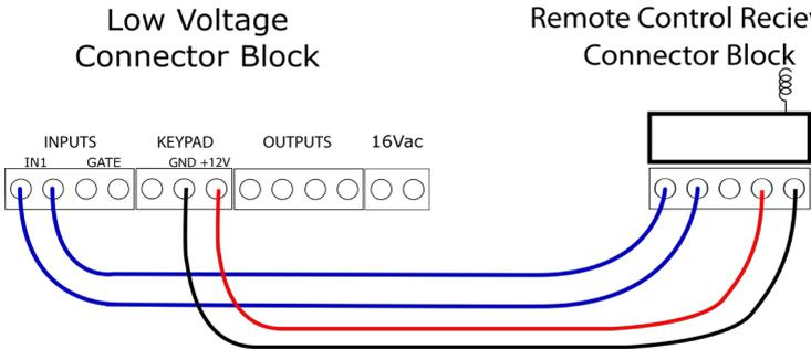
*Remote Control Receiver Wiring Diagram*
