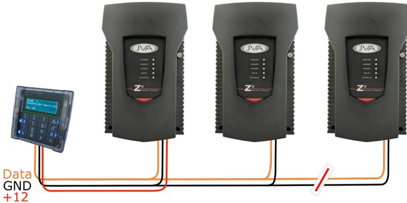
By disconnecting each Z-Series Energizer in turn from the keypad bus (shown in the above diagram) you can check to see how each Z-Series device behaves under comms fail conditions. This way, you can test to see that the relays have been configured correctly for comms fail. Once you are satisfied that each Z-Series device is configured correctly you can begin to wire them to the real fence.
