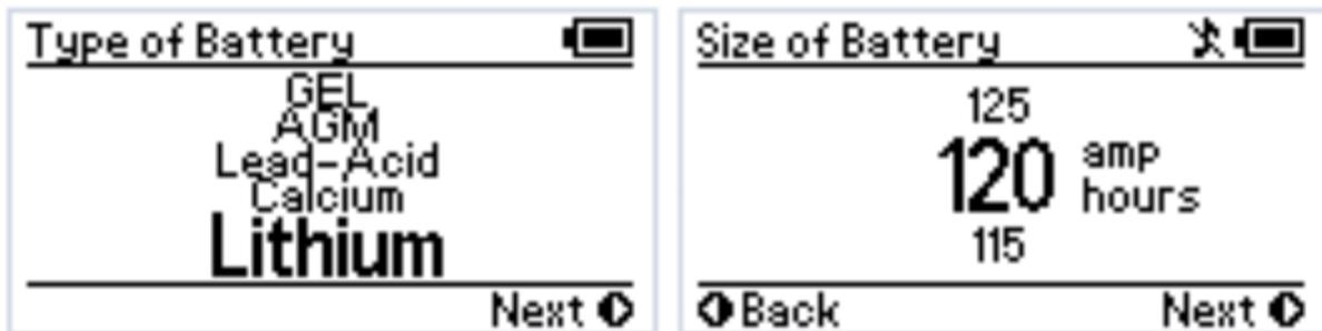
Secondly, the Manager needs to fully charge the battery. It does this so that it knows the battery has a full state of charge to use as a reference point for calculations on time till full or flat, and display its state of charge correctly. This process is displayed as "Calculating" on the remote.
