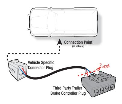
For use with the **Tow-Pro Classic** Electric Trailer Brake Controller (EBRHV2):
