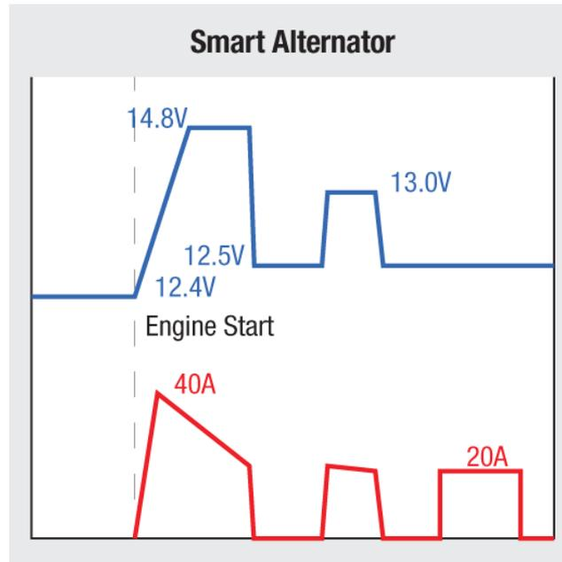
A. Engine is not running, relatively low open circuit voltage of the start battery approx. 12.4V, as the system does not aim to achieve a full state of charge in the start battery. Specific battery types are used in this application in order to achieve good performance and service life when operating at partial charge for starter operation.
