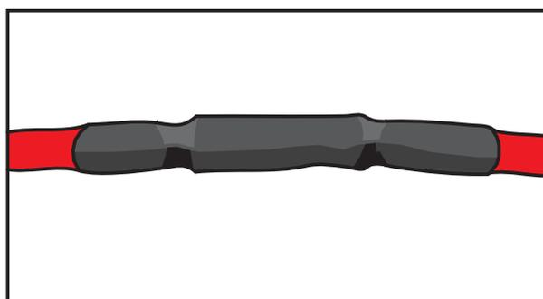
Wait for the butt splice to cool, slip heatshrink over the joint and heat.
