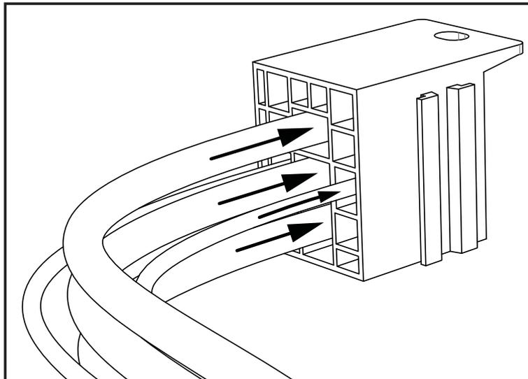
Diagram 4 - Inserting the wires into the relay base
