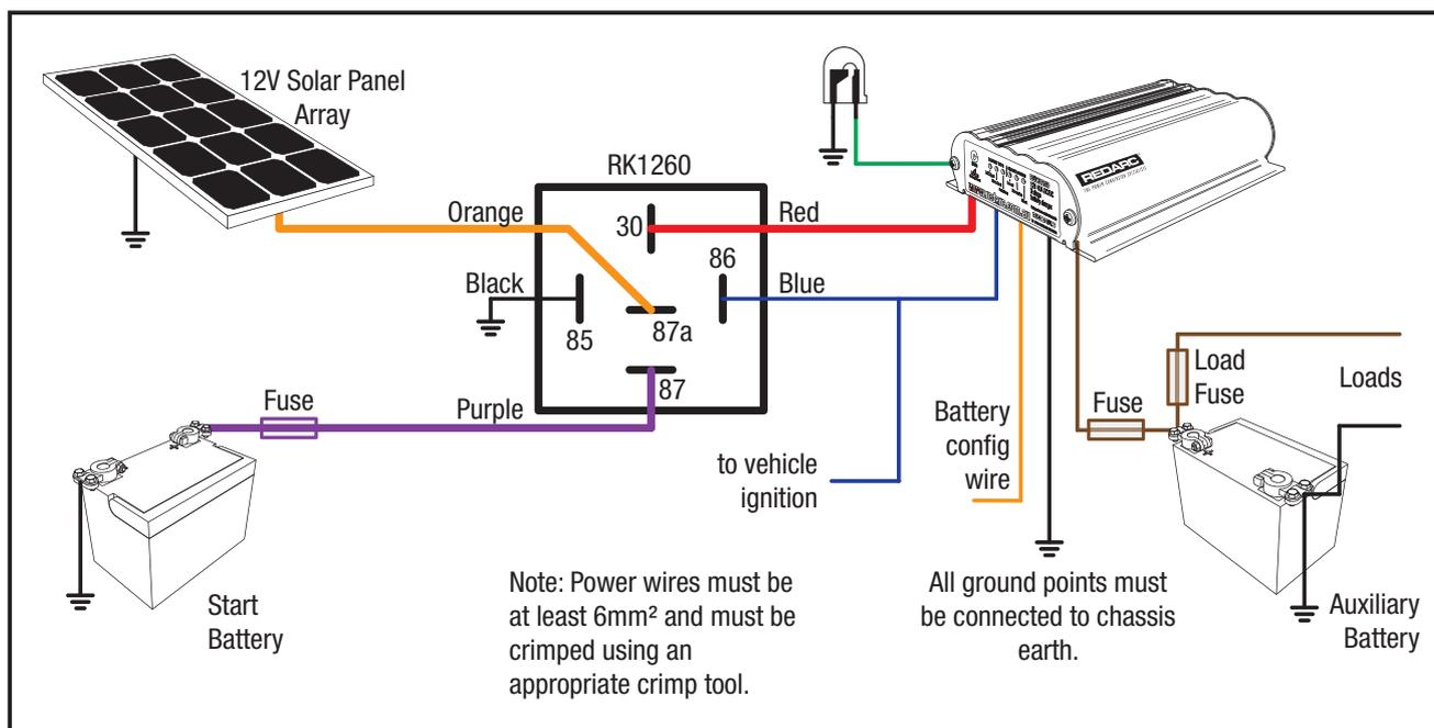
Diagram 2 - Wiring the RK1260
