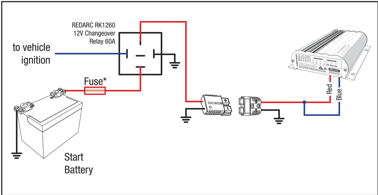
Diagram 2 - Wiring the RK1260
