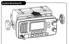
To Mount The Transceiver **On Almost Any Flat Surface:**
