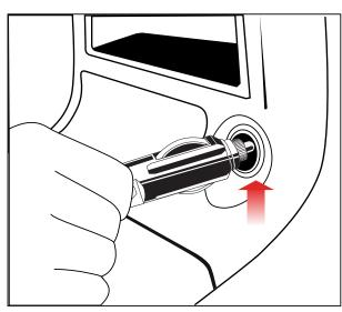
2 Depending on your vehicle, push the START button to Accessory mode or turn the ignition switch to the Accessory position
