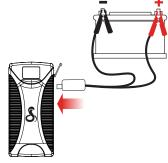
Disconnect the jumper cable from the Jump Starter 1000A and then from the battery
