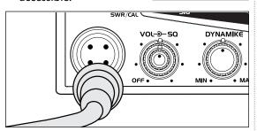
Attach the 4-pin microphone cable to receptacle on front of unit and install unit in bracket securely.
