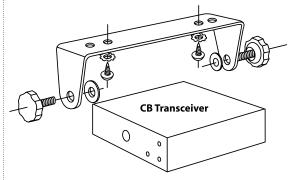
2 Drill the holes and secure the bracket.
