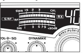
• The S/RF-SWR-CAL switch must be in the S/RF setting to read the meter.
