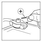
**5.** Connect the red wire marked "BATT" (+) directly to the positive side of the battery or to a connection on the fuse box that is always on.
