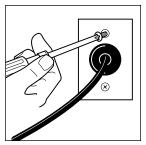
6. Connect the black leader marked "Ground" to the negative side of the car, usually the chassis. Any other location with good electrical contact (paint removed) will also work
