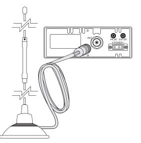
Connect the antenna cable plug to the receptacle marked "ANT" on the back of the unit.
