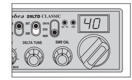
• Switch to BRT or DIM to control the brightness of the channel indicator and multi-function meter for day or nighttime driving.
