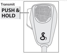
• Push and hold the mic button to transmit. The transmitter is now activated. When transmitting, hold the microphone two inches from your mouth and speak in a clear, normal voice. *Release* to receive.
