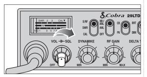
Rotate the On/Off Volume knob clockwise. The green RX/TX LED will be illuminated.
