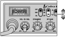
• When *switched* to • ANL the Automatic Noise Limiter is activated. This helps reduce noise created by the vehicle's electronics.
