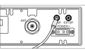
• Connect an external PA speaker to the PA jack on the rear panel.
