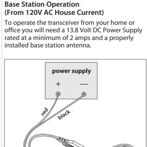
Simply connect the red (+) and black (-) leads of the transceiver to the corresponding terminals of the power pack.
