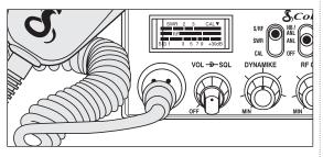
Attach the 4-pin microphone cable to the connector on the front of the radio and install the microphone on bracket securely.
