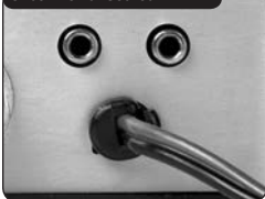
Check Fuses in DC Power Cord
