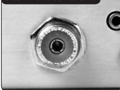
Check Antenna Connection
