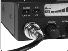
Check Antenna Connection
