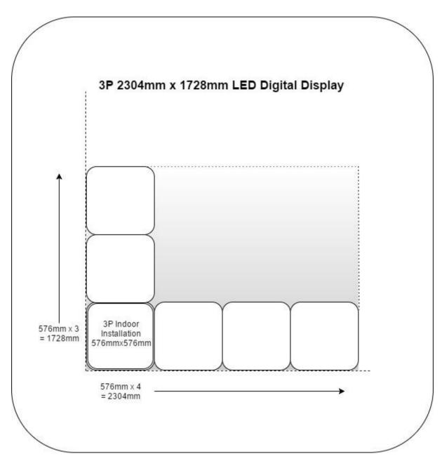
Once you have decided on the number of panels, you will need to find an appropriate sender box. To do this, find the total number of pixels for the LED Digital Display by referring back to the price list and finding the total number of pixels per panel (eg 192x192=36864) and then multiply that by the total number of required.
