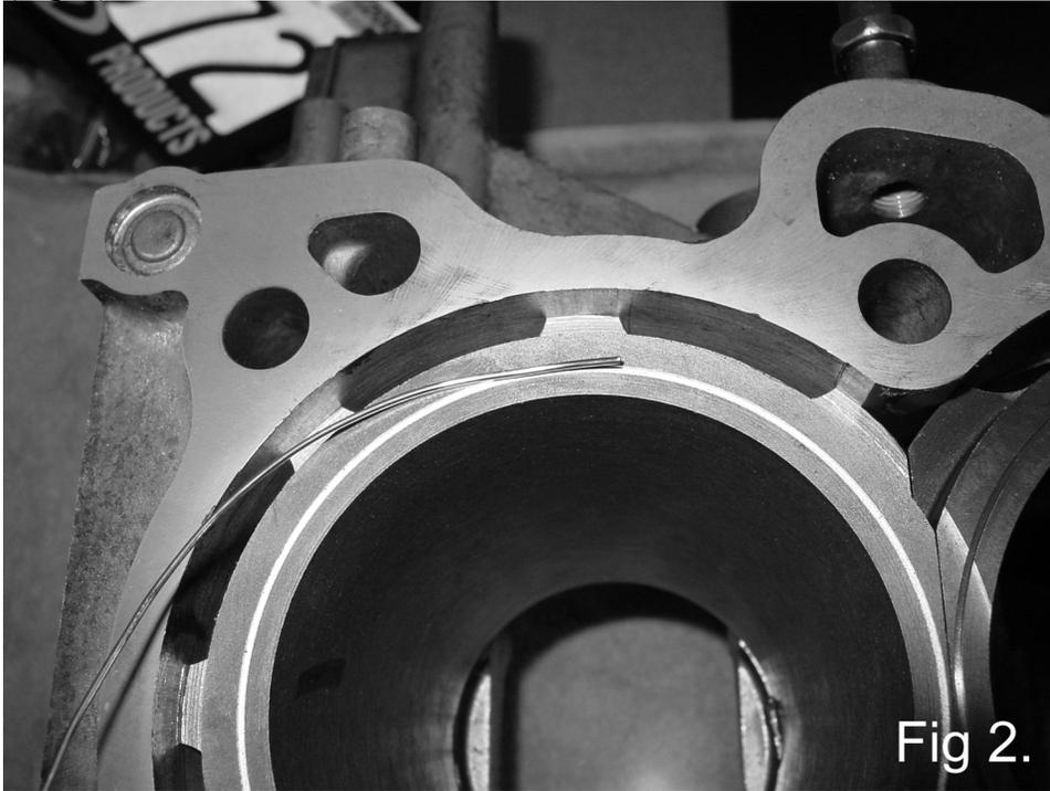
5. Using the butt end of the wooden handle hammer, *GENTLY* tap the wire into place. ( Fig 3 ) Continue tapping all the way around the bore.
