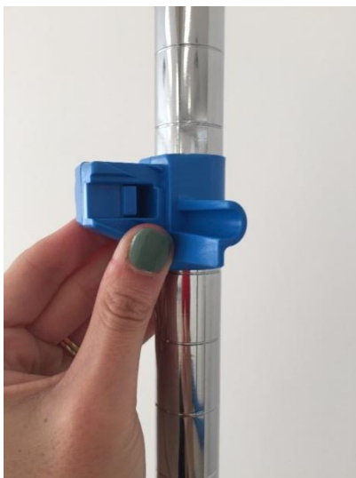
5. Slide the knuckle down post until the locating line on the knuckle locates into the groove on the post then close the knuckle around the post. Make sure the stopper on the knuckle faces inward.
