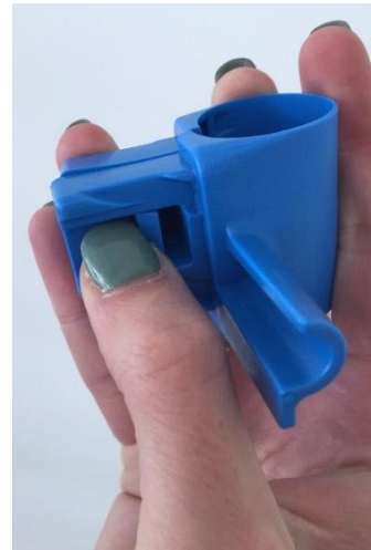
2. Open the knuckle by pushing the clip on the knuckle's side back until it releases.
