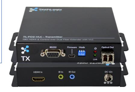
The TL-FO2-VLC is an HDMI 2.0 (18G signal) with HDCP 2.2 support fiber optic extender set that can reach up to 10km over a duplex fiber optic cable with common LC terminations. The unit supports HDMI video resolutions up to 4K@60, HDR video, IR or RS232 pass-through controls and multichannel audio. Integrated mounting ears are included on both the Tx and Rx units.
