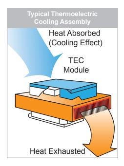
DBK Thermoelectric Coolers use the Peltier effect to provide compact and reliable solid state cooling. The application of DC voltage to the TEC creates a heat pump, which transfers heat from one side to the other, making one side cold and the other side hot. The use of heat sinks and fans produces a system which optimises the thermal transfer for cooling electrical enclosures.
