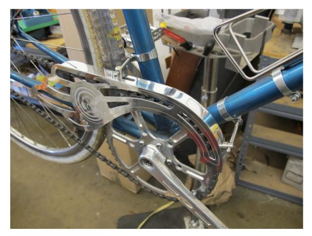
Adjust chain guard horizontally along stays. The inner side of the chain guard should be very close to the chain ( $\sim$ 2mm) in order to provide enough crank arm clearance. Adjust front eyelet bolt first, positioning the front of the chain guard the appropriate distance from the chain and then tightening that eyelet bolt down. Adjust the rear eyelet bolt in the same manner.
