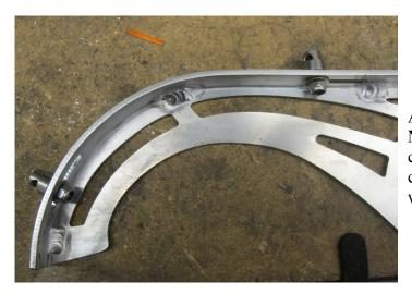
Attach eyelet bolts to chain guard. **Note:** the cupped washer goes on top side of chain guard, flat washers go on underside of chain guard. Use nylock nuts, which are nuts with a black nylon ring on the end.
