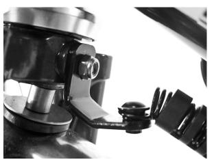
The bracket should be fastened to the fork crown as shown.
