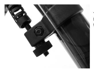
You'll secure the adjustment rod with the big knurled nut. Make sure the stepped side faces the front of the bike.
