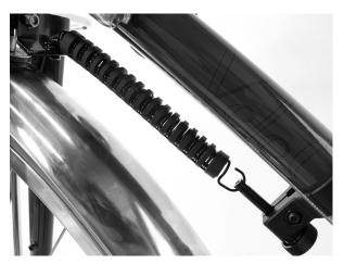
When you're finished, it looks about like this. Adjust the tension by sliding the clamp before tightening it down.
