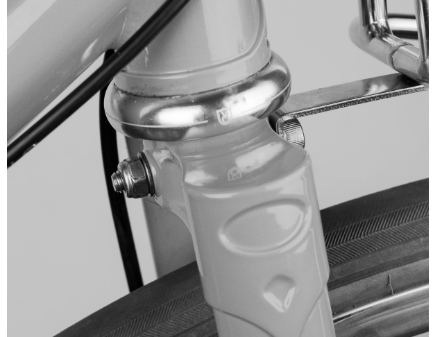
Bend is face up for cantilever brakes.
