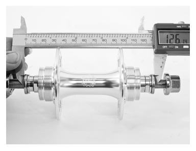
Use the two thin spacers for 126mm. Be sure to always put the same spacers on each side. Just remove the axle nuts and slide the spacers down the axle. You don't need to remove the axle locknuts!
