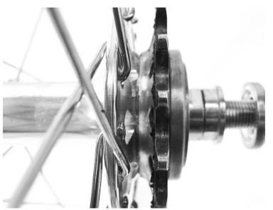
When you thread the sprocket and lockring on, it should be flush against the hub. Try to unscrew the sprocket (counterclockwise) - if the sprocket is thick enough, it will not unscrew because the lockring will be holding it in place.
