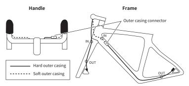
\*If you want to put the outer connector inside the frame, you must have a hole of 6.6mm or more.
