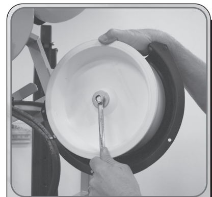
Figure 9 Hold wheel while loosening bolts.
