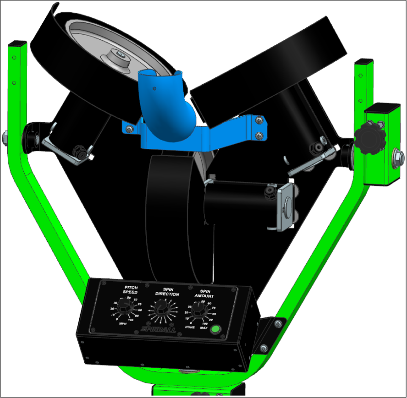
Figure 3: Ball feed ramp installation
