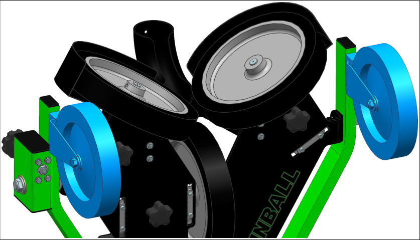
Figure 4: Transport wheel installation
