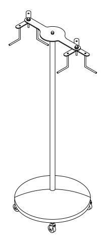
Net storage winder shall be capable of providing tangle free storage of two official volleyball nets in a vertical position. Net winding apparatus and riser pole shall be mounted to a 24" diameter dome shaped base fitted with 3 non marking casters. Entire assembly shall have a gray powder coated finish and weigh approximately 70#.
