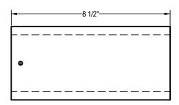
Sleeves are constructed of extruded aluminum tubing with an approximate inside diameter of 3" and outside diameter of 4". Suitable for installing a 3" diameter volleyball post in a 4" diameter socket. The sleeve length is approximate 8 1/2". Two 1/4" diameter threaded holes allow setscrews (provided) to attach the sleeve to either the 3" pole or to the inside diameter of the 4" floor socket or can be used without attachment.
