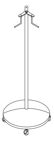
Net storage winder shall be capable of providing tangle free storage of one official volleyball net in a vertical position. Net winding apparatus and riser pole shall be mounted to a 24" diameter dome-shaped base fitted with 3 non marking casters. Entire assembly shall have a gray powder coated finish and weigh approximately 70#.
