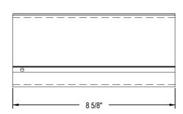
Sleeves are constructed of extruded aluminum tubing with an approximate inside diameter of 3 1/2" and outside diameter of 4". Suitable for installing a 3 1/2" diameter volleyball post in a 4" diameter socket. The sleeve length is approximate 8 1/2" Three 1/4" diameter threaded holes allow setscrews (provided) to attach the sleeve to either the 3 1/2" pole or to the inside diameter of the 4" floor socket or can be used without attachment.
