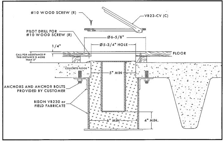
Only if the socket assembly wants to float in the hole, attach brass floor plate to wood floor using the wood s crews (R) provided. It is best to drill a small pilot hole into the wood to avoid cracking.
