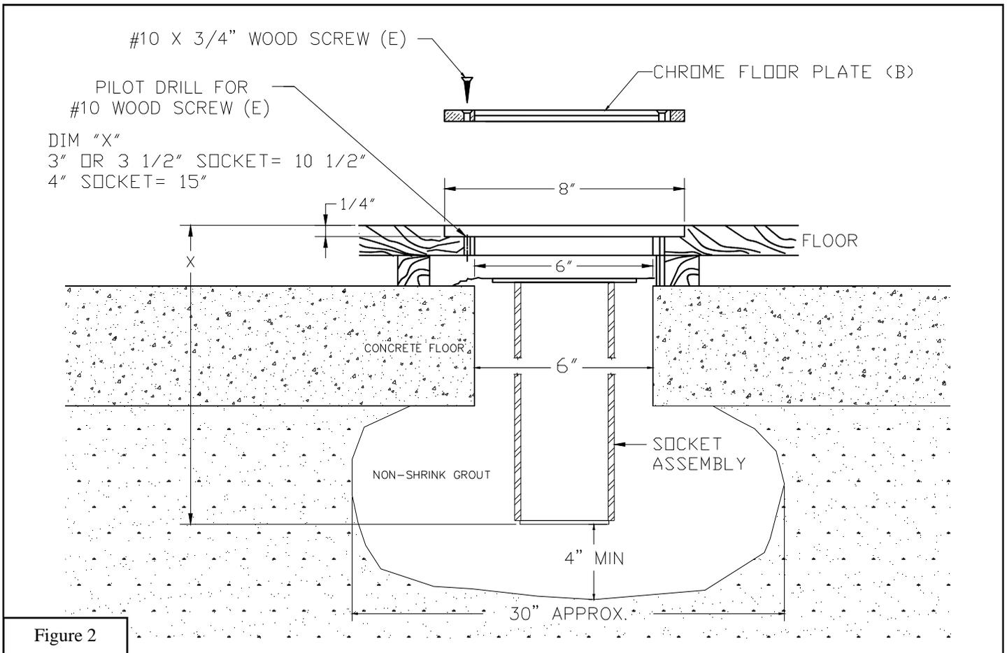
6. Insert the *Chrome Floor Plate (B)* into the routed floor pocket to insure proper fit. Use *Lid Key (K)* to lift and rotate the *Chrome Floor Plate (B)* lid so that the rotated lid is located outside the volleyball court and 180 degrees from the ultimate position of the net. Pre-drill an 1/8" pilot hole through the center of the 6 holes countersunk in the *Chrome Floor Plate (B)* to allow easy installation of the #10 X 3/4" *Wood Screws (E)* provided. See Figure 1.
