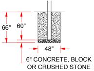
NOTE: SUGGESTED FOOTING, CHECK LOCAL BUILDING CODES BEFORE STARTING THE FOOTING, AS BUILDING CODES MAY VARY. LOCAL BUILDING CODES SHOULD BE ADHERED TO IF REQUIREMENTS ARE GREATER THAN THOSE OUTLINED HERE.
