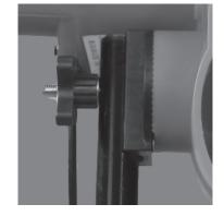
C: Slide Flat Washer (1st) and Lock Washer (2nd) on to the Long Bolt, then tighten the Knob on to Long Bolt until machine is placed in the desired pitching position.
