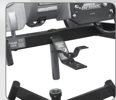
Figure 8D Lift the throwing head completely out of the undercarriage.
