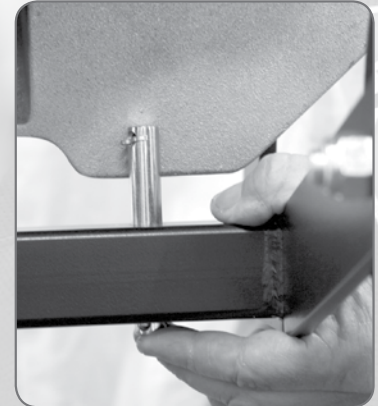
Figure 8B Hold frame lock all the way up until the throwing head is held tightly against the frame lock pin.
